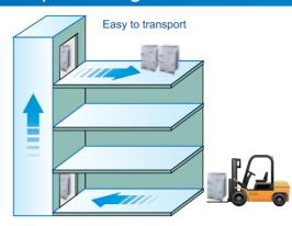
Compact size and light weight design minimizes the installation footprint, reduces the installation floor load, and is easier for transportation. For some projects the units can even be transported through the elevator or forklift, reduce access problem at the jobsite.
